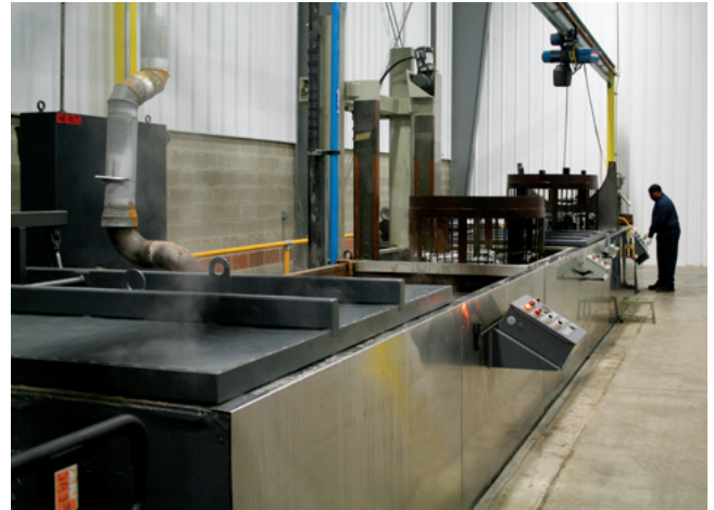
Figure 4 - Batch Process Vacuum Impregnation System.
