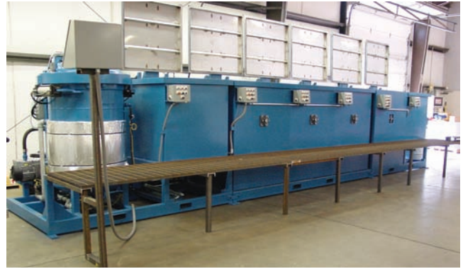
Figure 6 – The top loading or batch system is the most common type of impregnation system in practice today.
